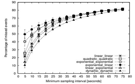
Figure 3. Percentage of missed events vs minimum sampling interval for Bluetooth sensor.
