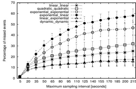
Figure 5. Percentage of missed events vs maximum sampling interval for Bluetooth sensor.
