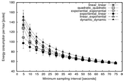
Figure 4. Energy consumption vs minimum sampling interval for Bluetooth sensor.
